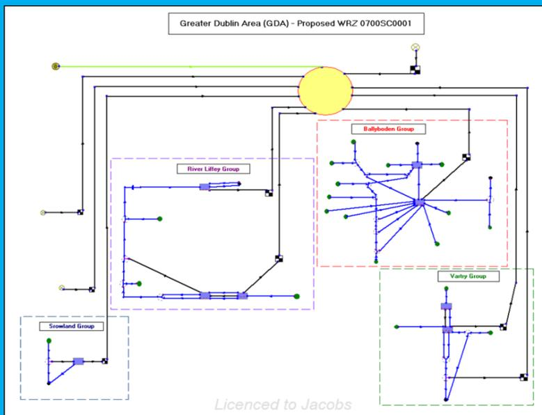
As the GDA WRZ is a complex network consisting of nine individual water supplies, the supply has been modelled using a water resource planning tool known as Aquator. The Aquator model enables us to assess the deployable output for the combined supplies for all weather conditions (normal, dry, drought and winter), for an appropriate level of service.
