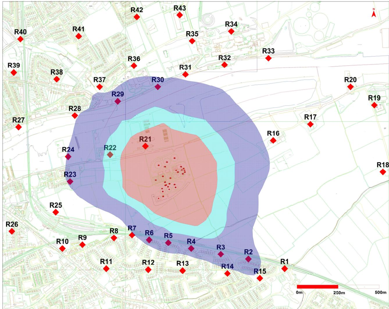
**Figure 7.6.** Predicted odour emission contribution of existing Drogheda WwTP odour sources for Model 4 to odour plume dispersal for an odour concentration of less than or equal to 1.50  $O_{uE}/m^3$  (blue), 3.0  $O_{uE}/m^3$  (cyan) & 5.0  $O_{uE}/m^3$  (red) for the 99.5<sup>th</sup> percentile of hourly averages for worst case meteorological year Dublin Airport 2019.
