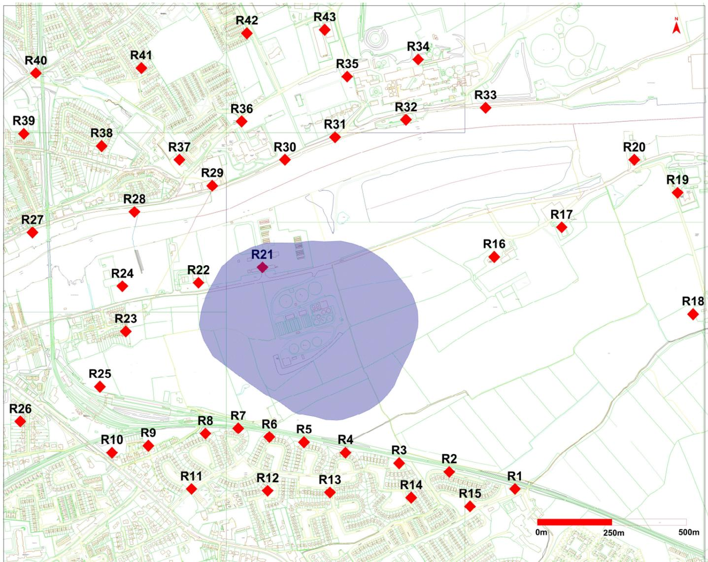
Figure 7.7. Predicted odour emission contribution of existing Drogheda WwTP odour sources for Model 5 to odour plume dispersal for an odour concentration of less than or equal to  $1.0 \text{ Ou}_E \text{ m}^{-3}$  (■) for the 98<sup>th</sup> percentile of hourly averages for worst case meteorological year Dublin Airport 2019.
