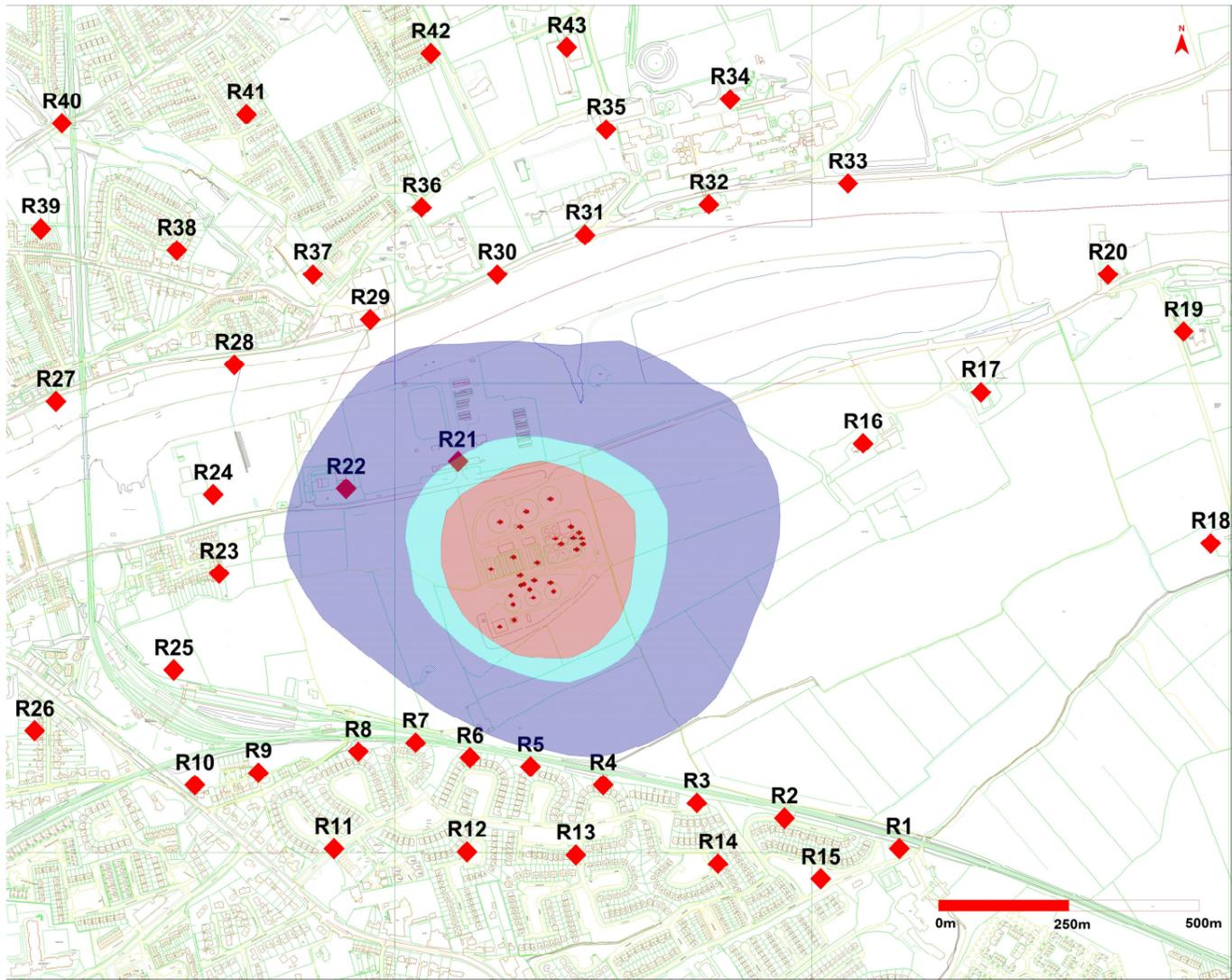
**Figure 7.5.** Predicted odour emission contribution of existing Drogheda WwTP odour sources for Model 3 to odour plume dispersal for an odour concentration of less than or equal to 1.0  $O_{uE}/m^3$  (blue), 3.0  $O_{uE}/m^3$  (cyan) & 5.0  $O_{uE}/m^3$  (red) for the 98<sup>th</sup> percentile of hourly averages for worst case meteorological year Dublin Airport 2019.
