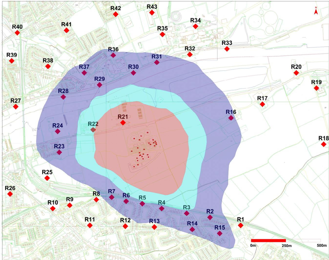
**Figure 7.4.** Predicted odour emission contribution of existing Drogheda WwTP odour sources for Model 2 to odour plume dispersal for an odour concentration of less than or equal to 1.0  $O_{uE}/m^3$  (blue), 3.0  $O_{uE}/m^3$  (cyan) & 5.0  $O_{uE}/m^3$  (red) for the 99.5<sup>th</sup> percentile of hourly averages for worst case meteorological year Dublin Airport 2019.
