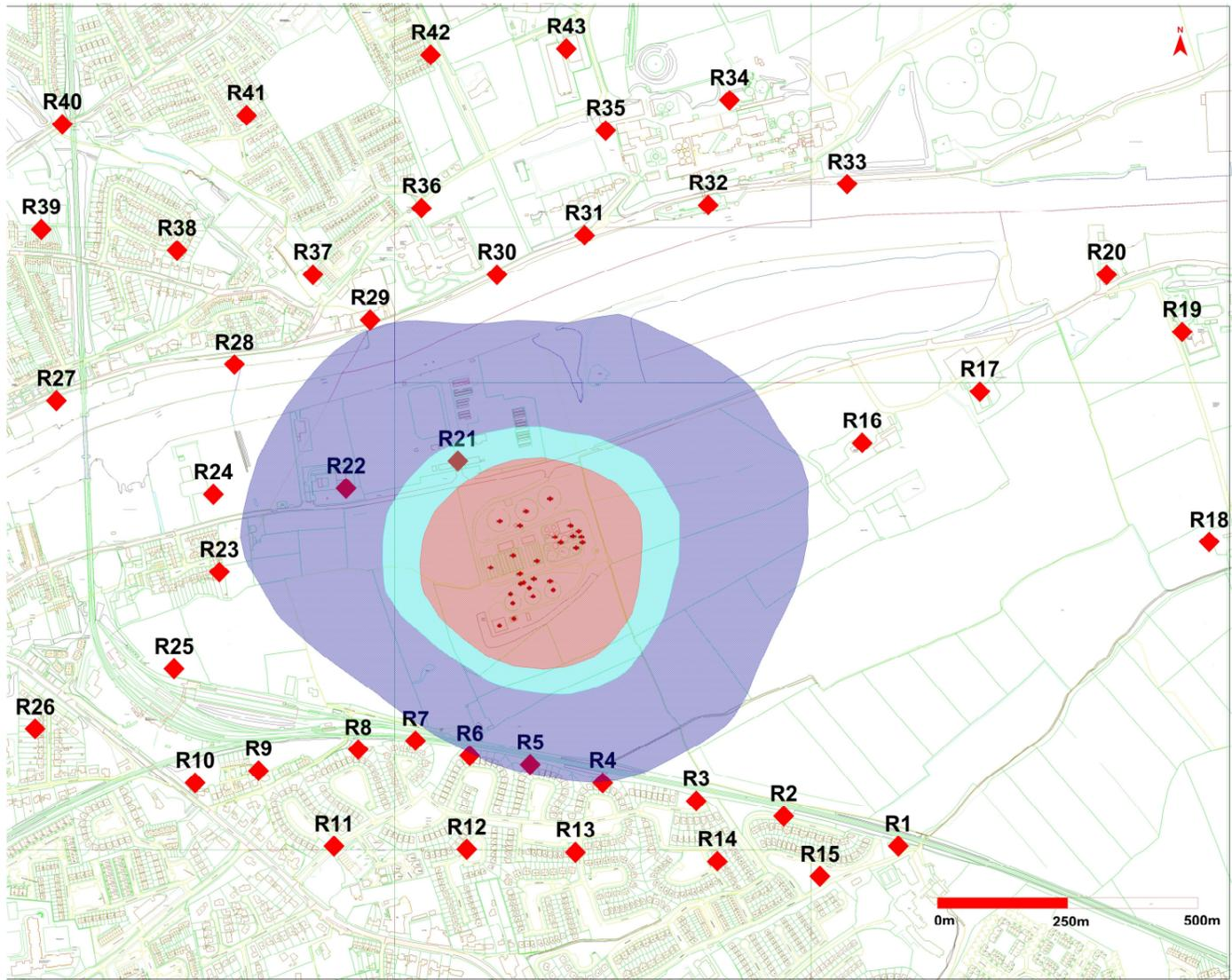
**Figure 7.3.** Predicted odour emission contribution of existing Drogheda WwTP odour sources for Model 1 to odour plume dispersal for an odour concentration of less than or equal to  $1.0 \text{ OuE/m}^3$  (blue),  $3.0 \text{ OuE/m}^3$  (cyan) &  $5.0 \text{ OuE/m}^3$  (red) for the 98<sup>th</sup> percentile of hourly averages for worst case meteorological year Dublin Airport 2019.
