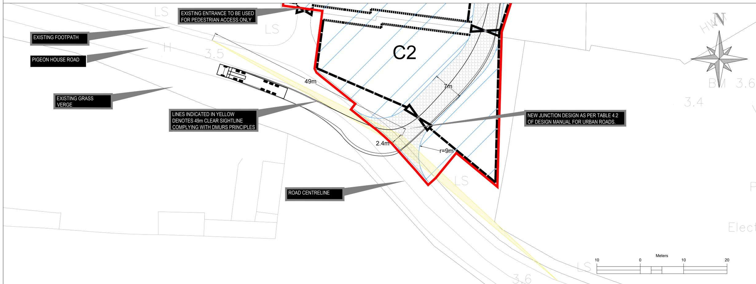
AUTOTRACK ANALYSIS FOR ARTICULATED VEHICLE EXITING COMPOUND C2
