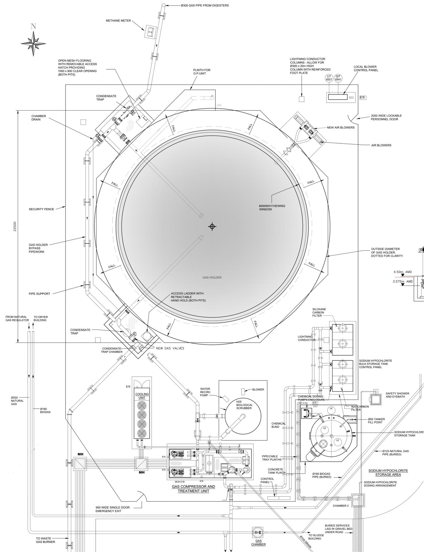
EXISTING PLAN LAYOUT OF BIOGAS STORAGE UNIT - RELOCATED
