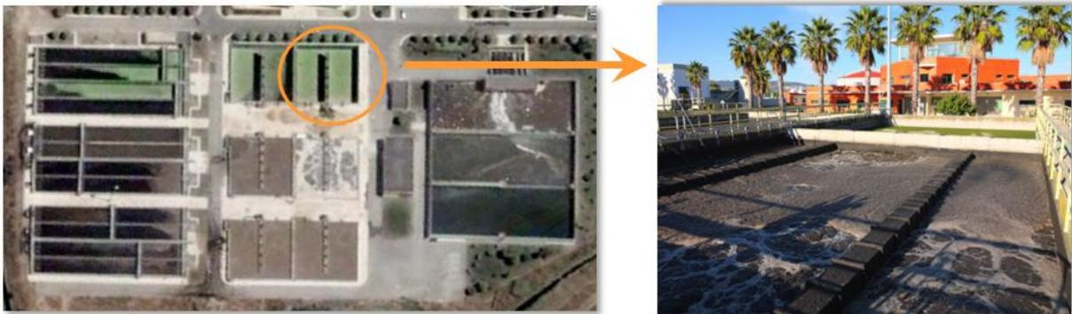
Figure 13. Conversion of reactor n°6 of Frielas WWTP to Nereda<sup>®</sup> technology.
