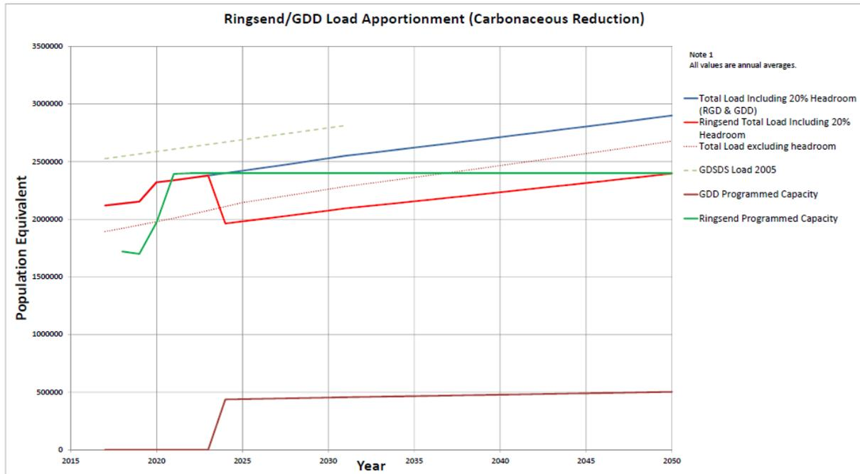
Figure 3-1: Historic and projected loadings for the Ringsend catchment (Carbonaceous reduction)
