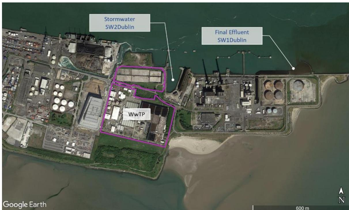
**Figure 4-1: Ringsend Wastewater Treatment Plant and storm overflow discharges**
