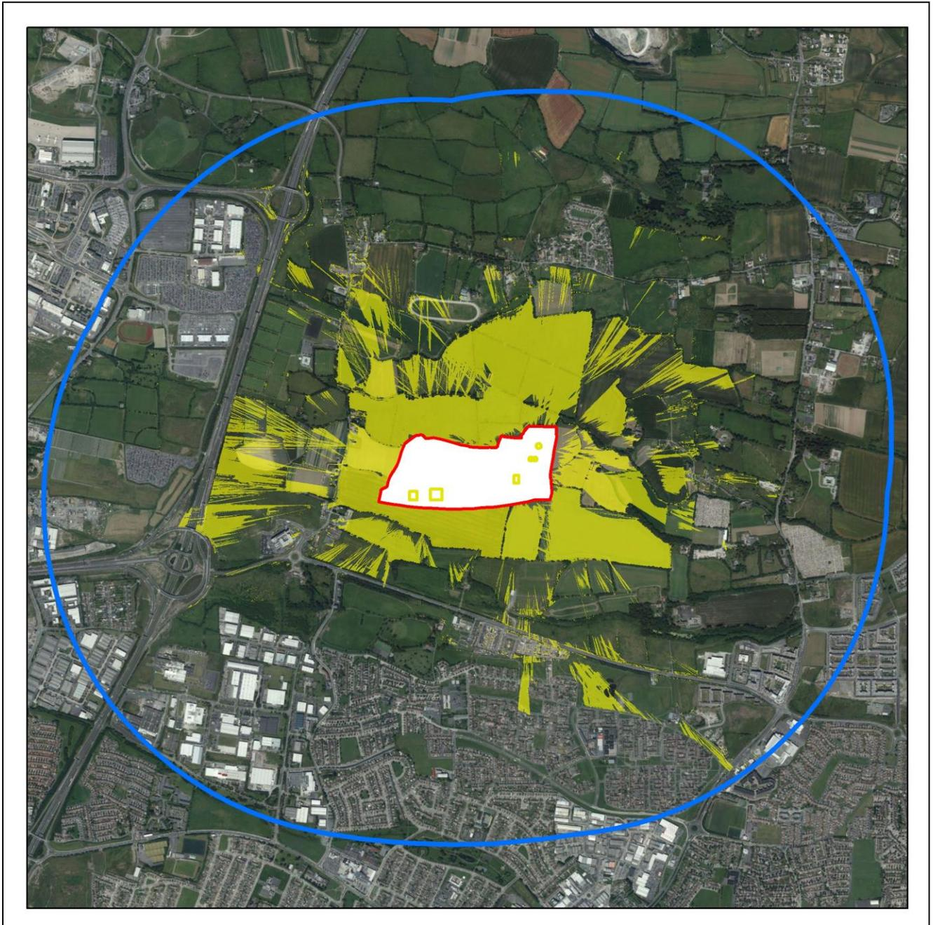
**Figure 10.2 – Digital Surface Model (DSM) based visibility map indicating from where in the surrounding landscape any part of the tallest potential structures (15m+) will be visible for ground-based receptors once existing screening is accounted for**
