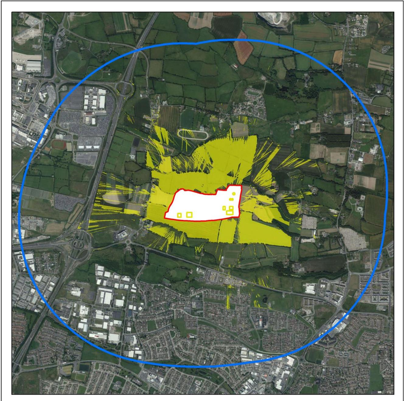
**Figure 10.3 – Digital Surface Model (DSM) based visibility map indicating from where in the surrounding landscape any part of the structures of 10m+ in height will be visible for ground-based receptors once existing screening is accounted for**
