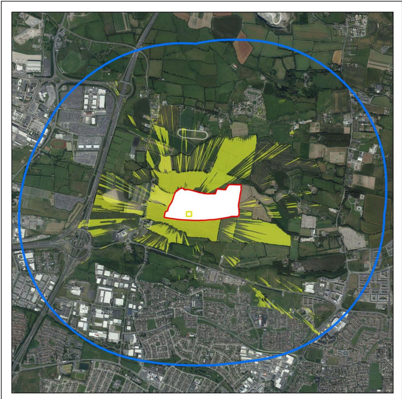
Figure 10.1 – Digital Surface Model (DSM) based visibility map indicating from where in the surrounding landscape any part of the tallest potential structure (18m) will be visible for ground-based receptors once existing screening is accounted for
