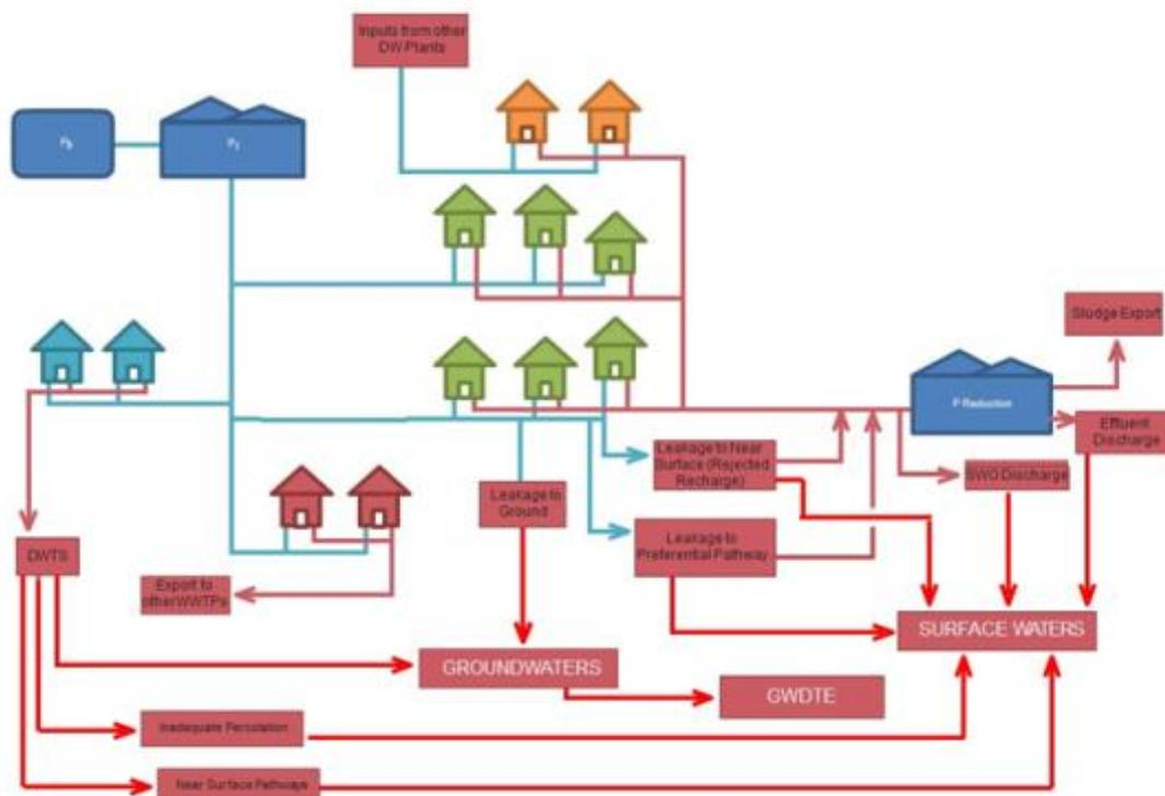
**Figure 5 Conceptual Model of P Transfer**
