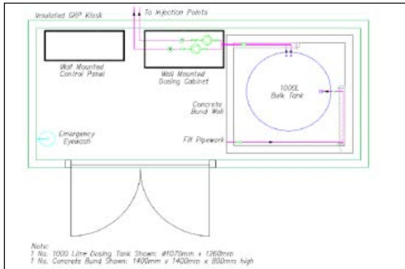
Figure 3 schematic of a bulk tank kiosk layout in H<sub>3</sub>PO<sub>4</sub> Installation with 500 litres < bulk storage ≤ 6,000 litres.
