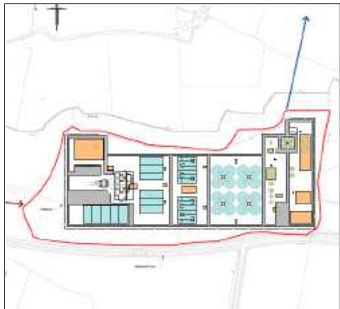
Figure 8.6 -WwTP Indicative Layout - Clonshagh
