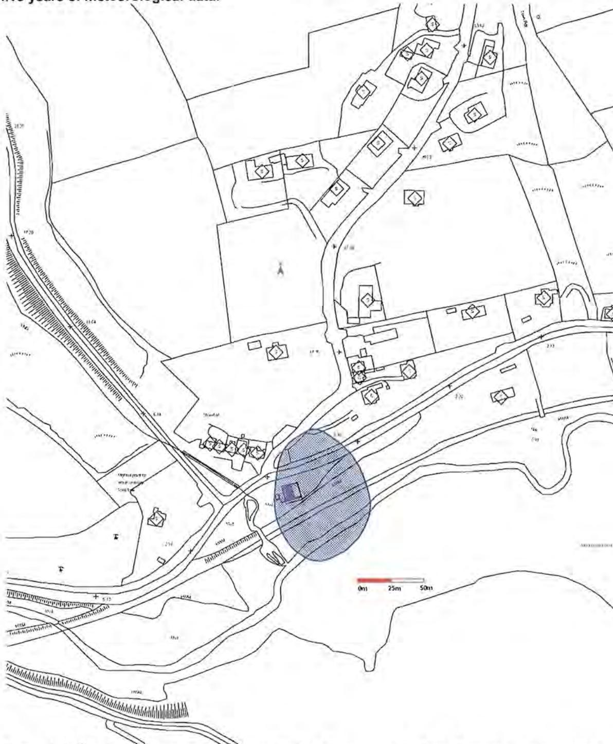
**Figure 8.5.** Predicted odour emission contribution of proposed Raffeen Pumping station operation with odour management protocols implemented to odour plume dispersal for Scenario 2 at the 98<sup>th</sup> percentile for odour concentrations  $\leq 0.10 \text{ Ou}_E \text{ m}^{-3}$  ( — ) for five years of meteorological data.
