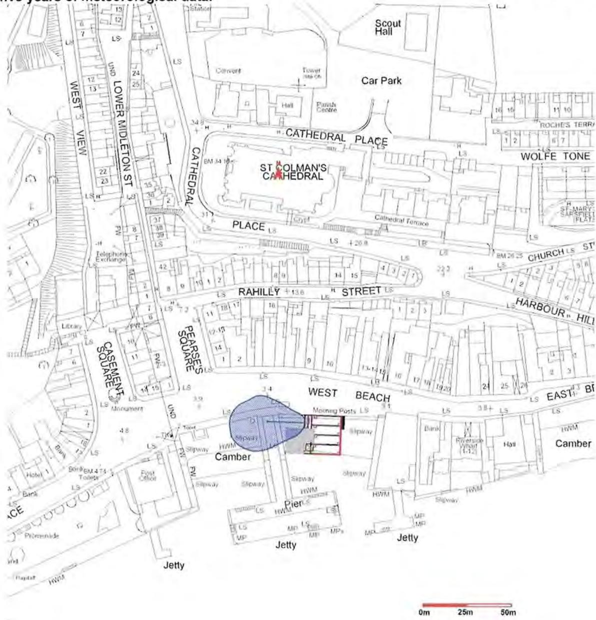
Figure 8.6. Predicted odour emission contribution of proposed West beach Pumping station operation with odour management protocols implemented to odour plume dispersal for Scenario 2 at the 98<sup>th</sup> percentile for odour concentrations  $\leq 0.30 \text{ Ou}_E \text{ m}^{-3}$  ( — ) for five years of meteorological data.
