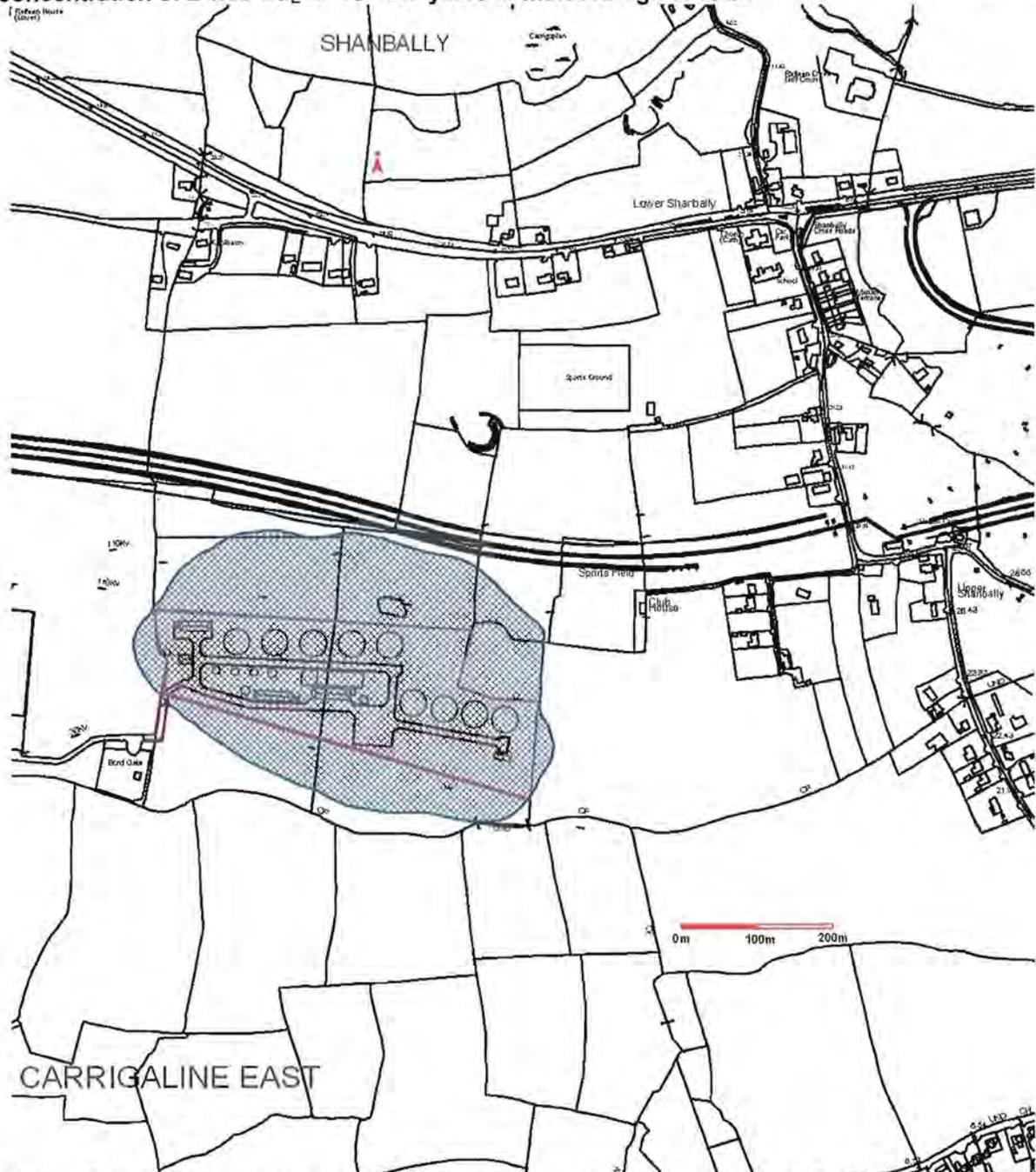
**Figure 8.1.** Predicted odour emission contribution of proposed overall Cork harbour WWTP operation with odour abatement protocols implemented to odour plume dispersal for Scenario 1 at the 98<sup>th</sup> percentile for odour concentrations  $\leq 1.5 \text{ Ou}_E \text{ m}^{-3}$  ( — ) for five years of meteorological data.
