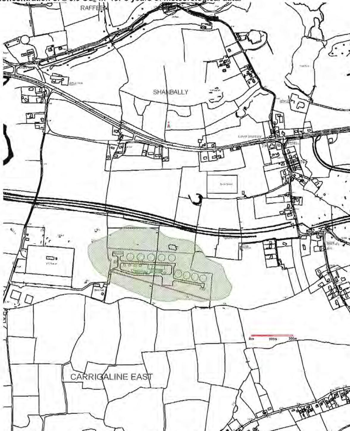
Figure 8.2. Predicted odour emission contribution of proposed overall Cork harbour WWTP operation with odour abatement protocols implemented to odour plume dispersal for Scenario 1 at the 99.5<sup>th</sup> percentile for odour concentrations  $\leq 3.0 \text{ Ou}_E \text{ m}^{-3}$  ( — ) for 5 years of meteorological data.
