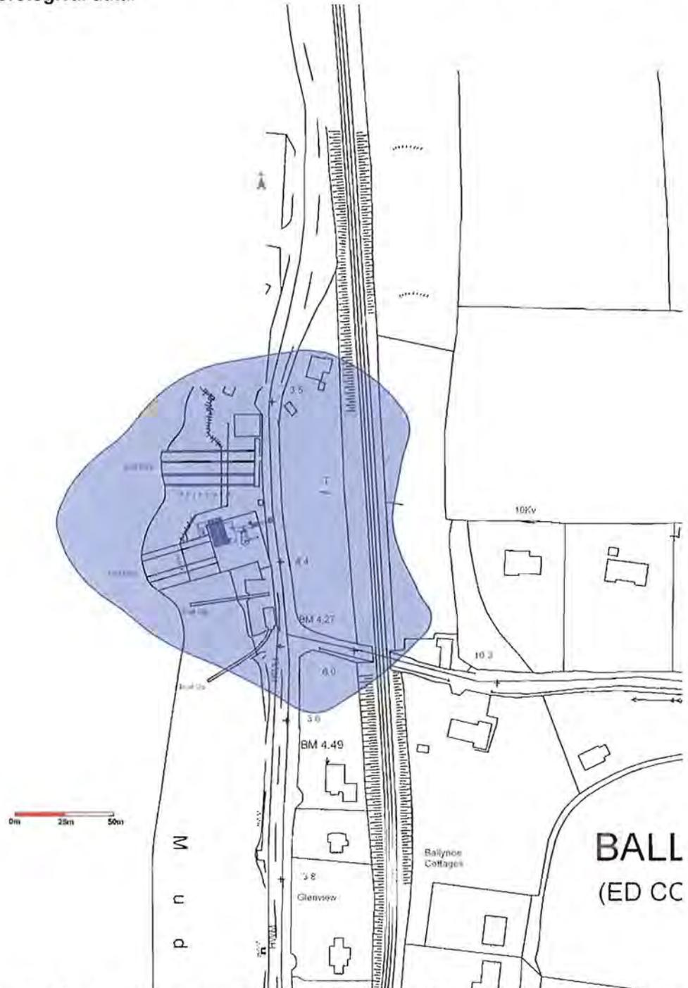
**Figure 8.9.** Predicted odour emission contribution of proposed Carraigaloe Pumping station operation with odour management protocols implemented to odour plume dispersal for Scenario 2 at the 98<sup>th</sup> percentile for odour concentrations  $\leq 0.10 \text{ Ou}_E \text{ m}^3$  ( — ) for five years of meteorological data.
