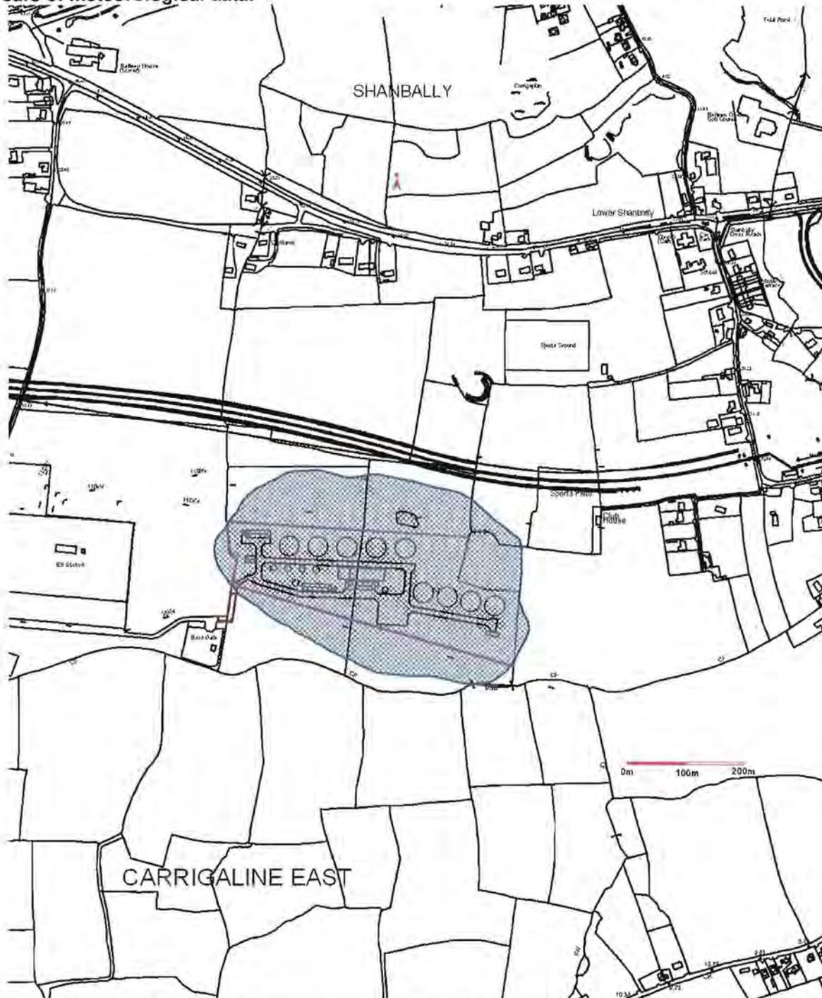
Figure 8.4. Predicted odour emission contribution of overall proposed WWTP to odour plume dispersal for grouped odour sources aeration tankage, Secondary settlement tankage and Storm water tankage for an odour concentration of less than or equal to  $1.50 \text{ Ou}_E \text{ m}^{-3}$  (—) at the 98<sup>th</sup> percentile of hourly averages for 5 years of meteorological data.
