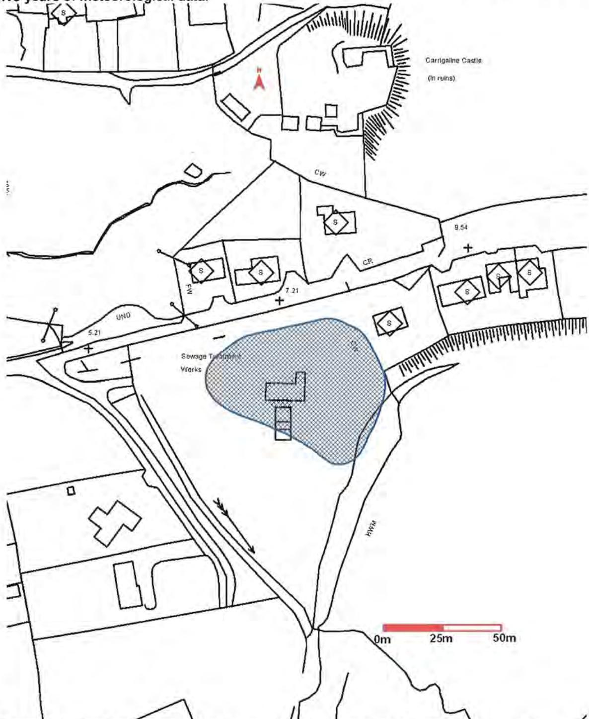
Figure 8.8. Predicted odour emission contribution of proposed Church Road Pumping station operation with odour management protocols implemented to odour plume dispersal for Scenario 2 at the 98<sup>th</sup> percentile for odour concentrations  $\leq 0.14 \text{ Ou}_E \text{ m}^{-3}$  ( — ) for five years of meteorological data.
