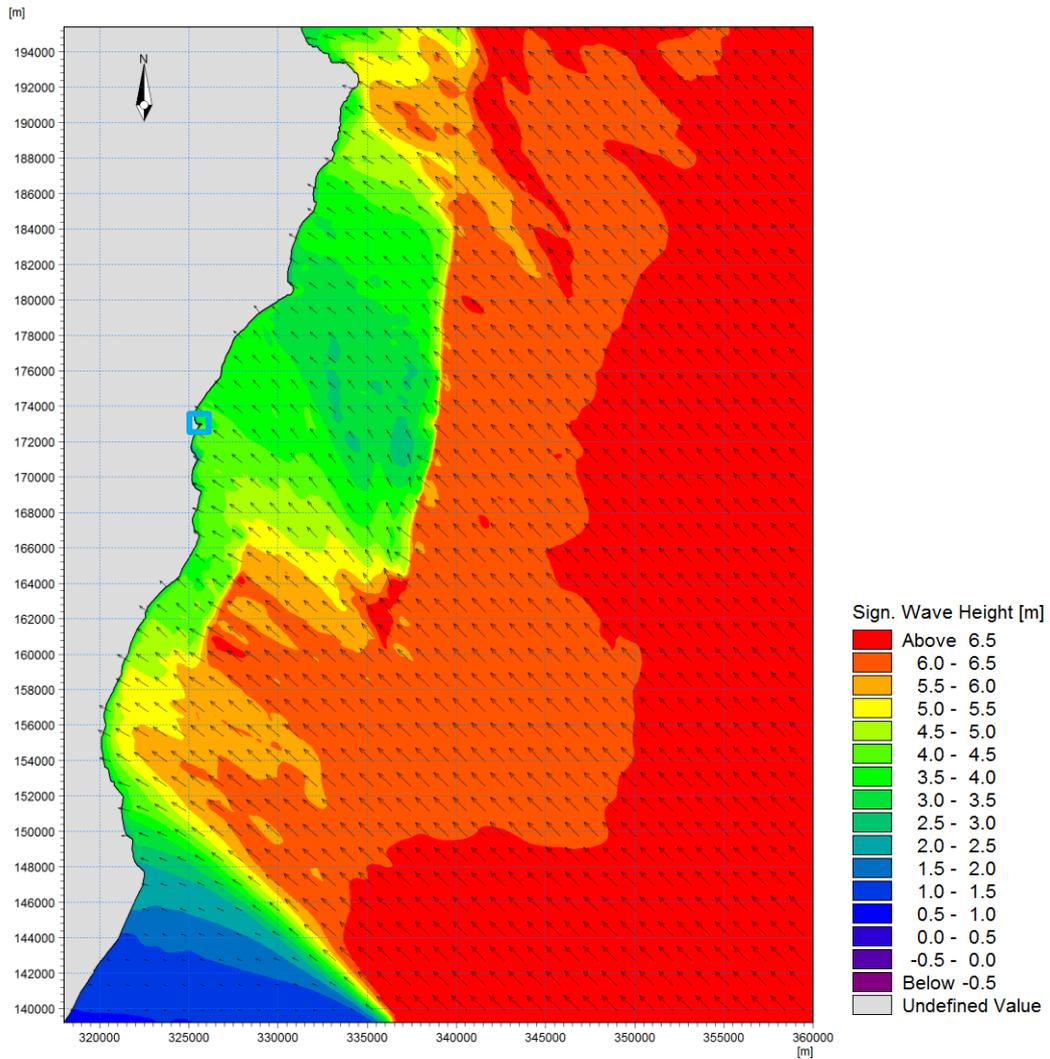
Figure 50: Wave height distribution with waves from the SE. Zoomed in on Arklow revetment site location.
