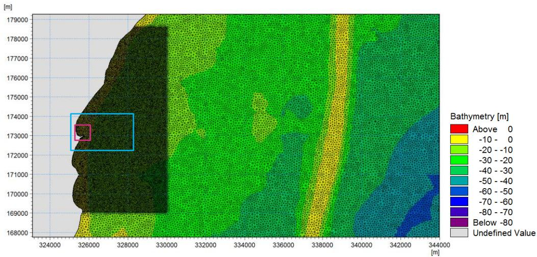
Figure 19: MIKE21-SW (high density) mesh at revetment location.
