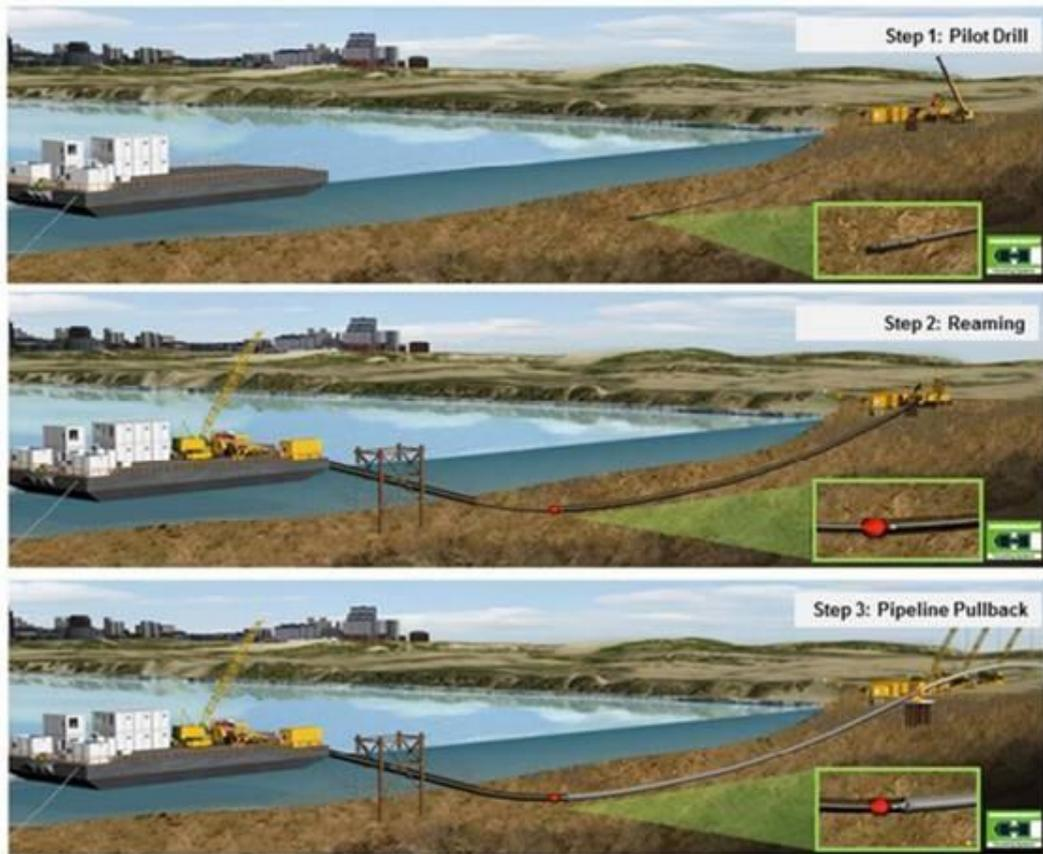
First, a drill rig would be positioned at a designated launch point (i.e. within the WwTP site), from which pilot boring would be carried out. The pilot boring would be undertaken to excavate along the alignment of the outfall.
