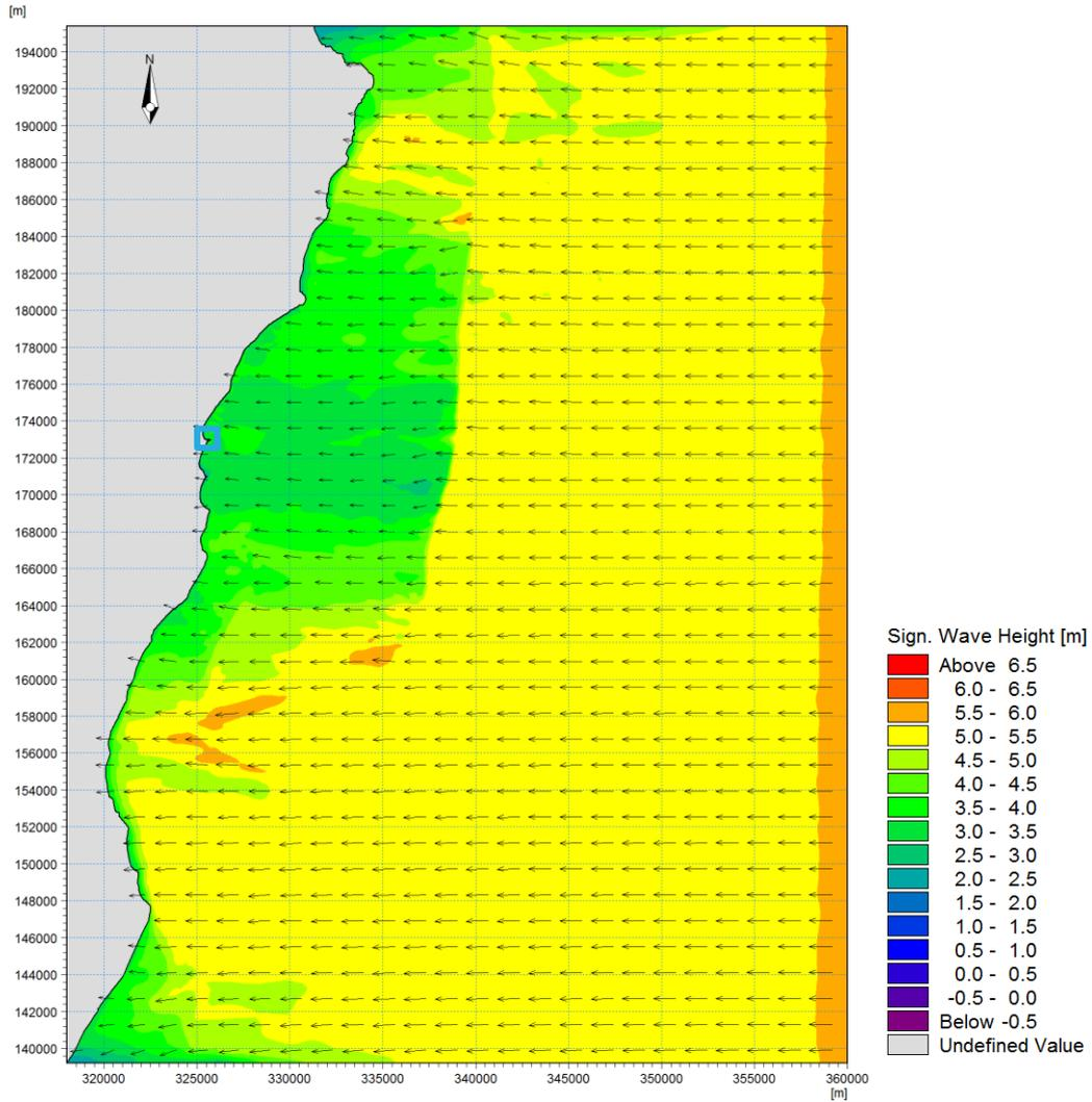
Figure 46: Wave height distribution with waves from the E. Zoomed in on Arklow revetment site location.
