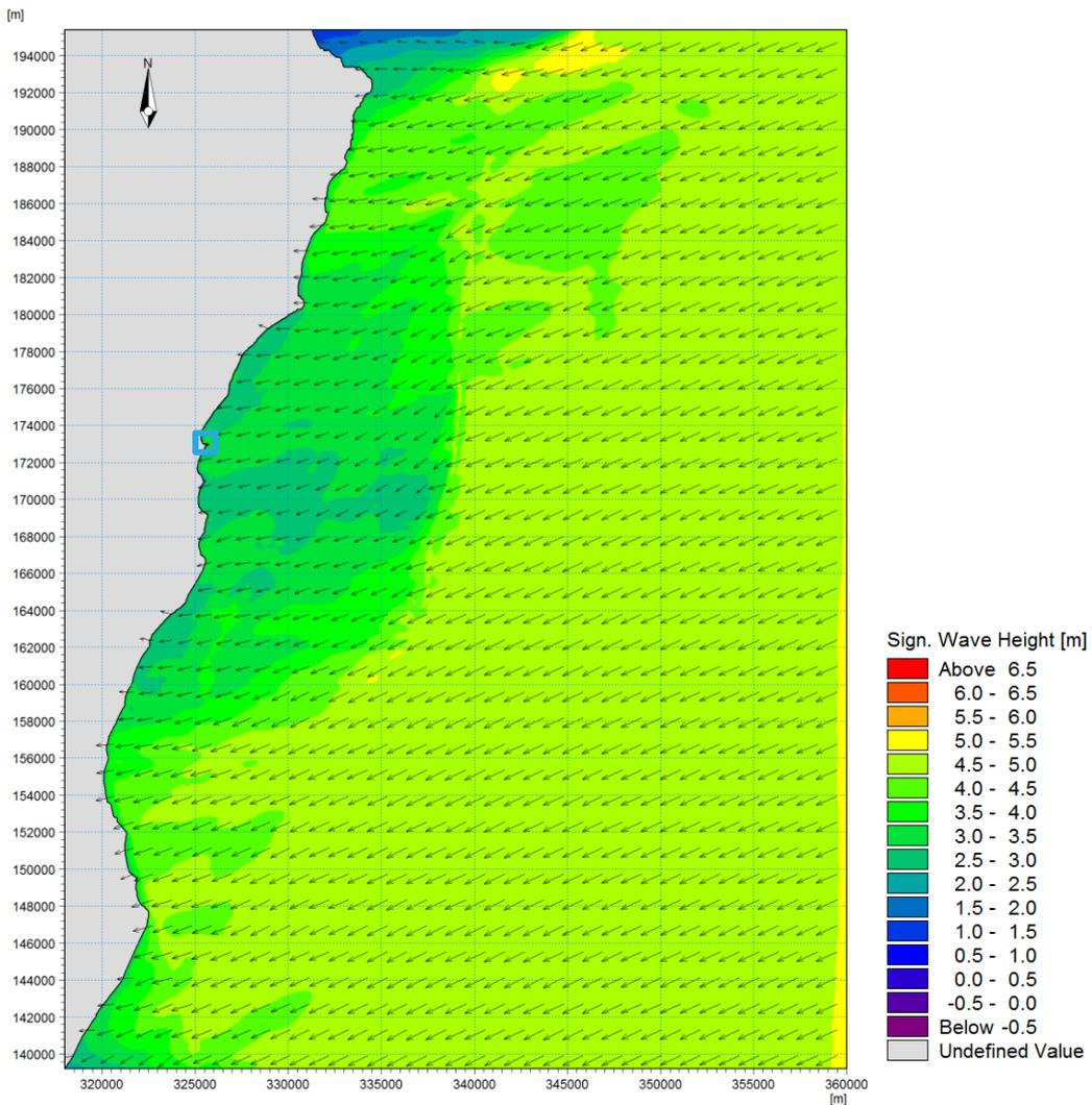
Figure 44: Wave height distribution with waves from the ENE. Zoomed in on Arklow revetment site location
