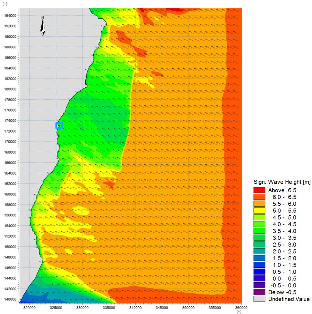
Figure 48: Wave height distribution with waves from the ESE. Zoomed in on Arklow revetment site location.
