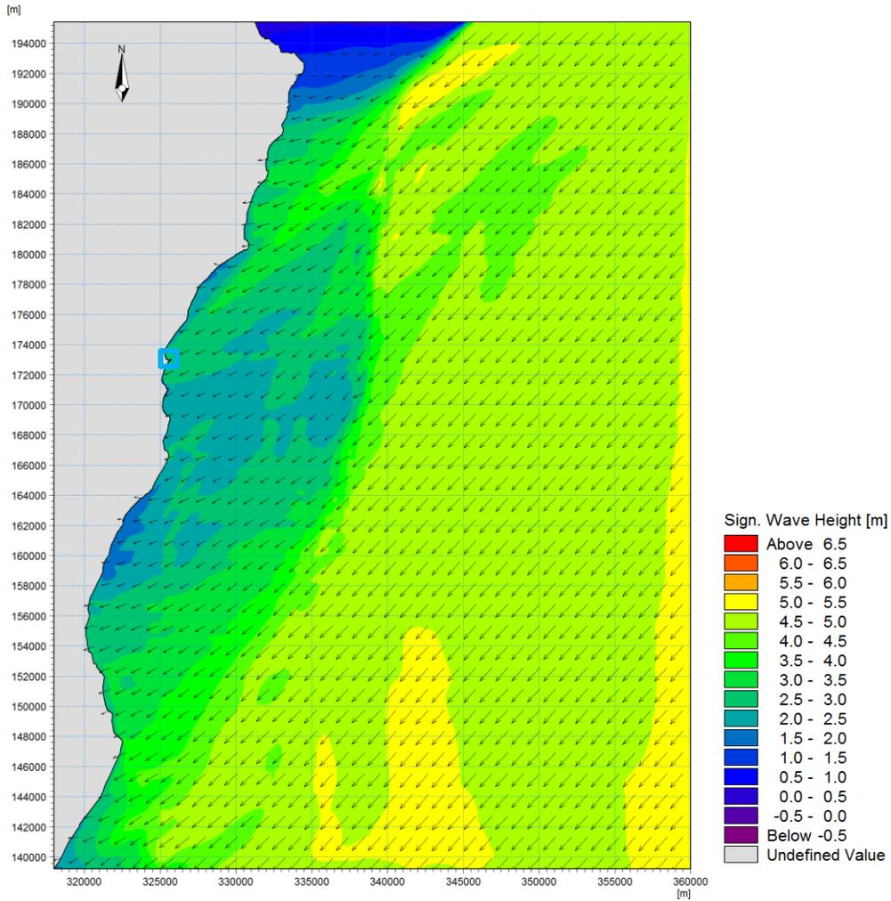
Figure 42: Wave height distribution with waves from the NE. Zoomed in on Arklow revetment site location.
