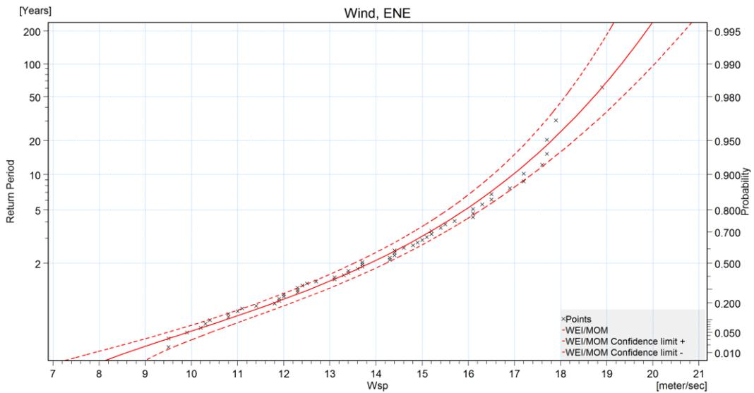
Figure 36: Extreme value analysis for the wind speed ( $W_{sp}$ ) and E.
