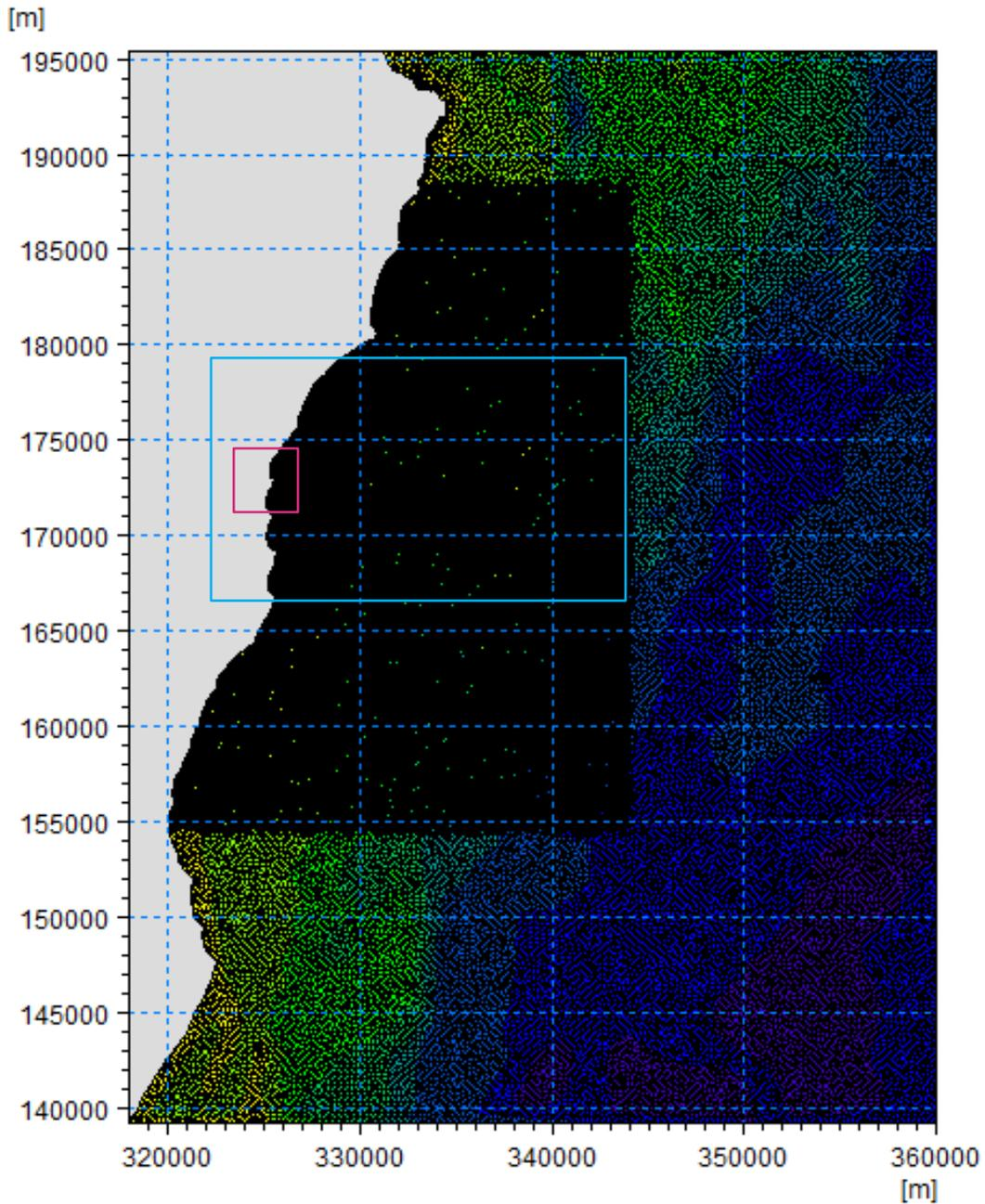
Figure 18: MIKE21-SW mesh (intermediate and high density). Blue square shows the boundaries of Figure 19.
