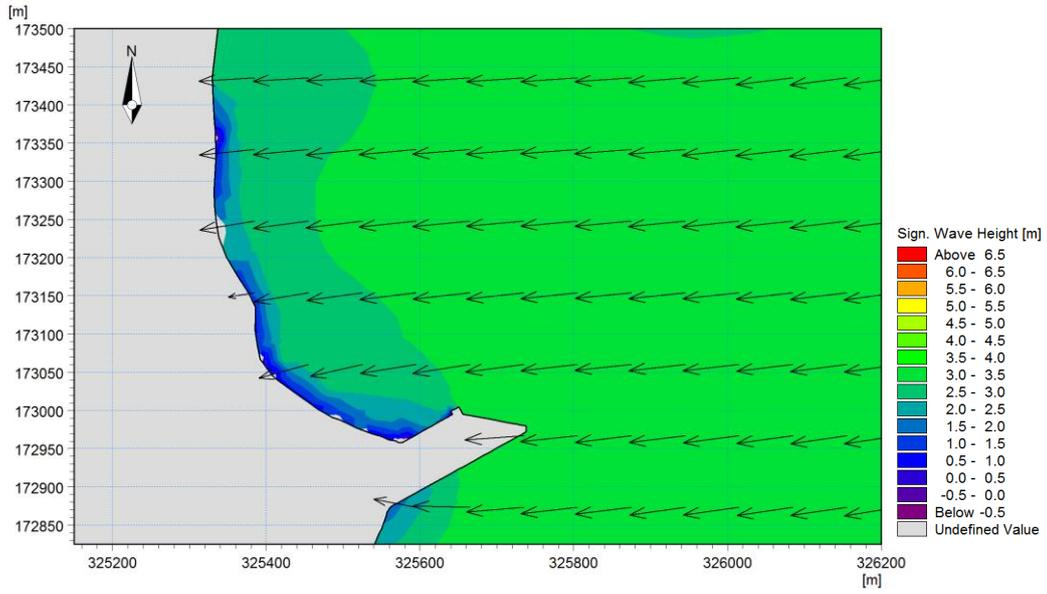
Figure 45: Offshore wave height distribution with waves from the E. Total computational domain.
