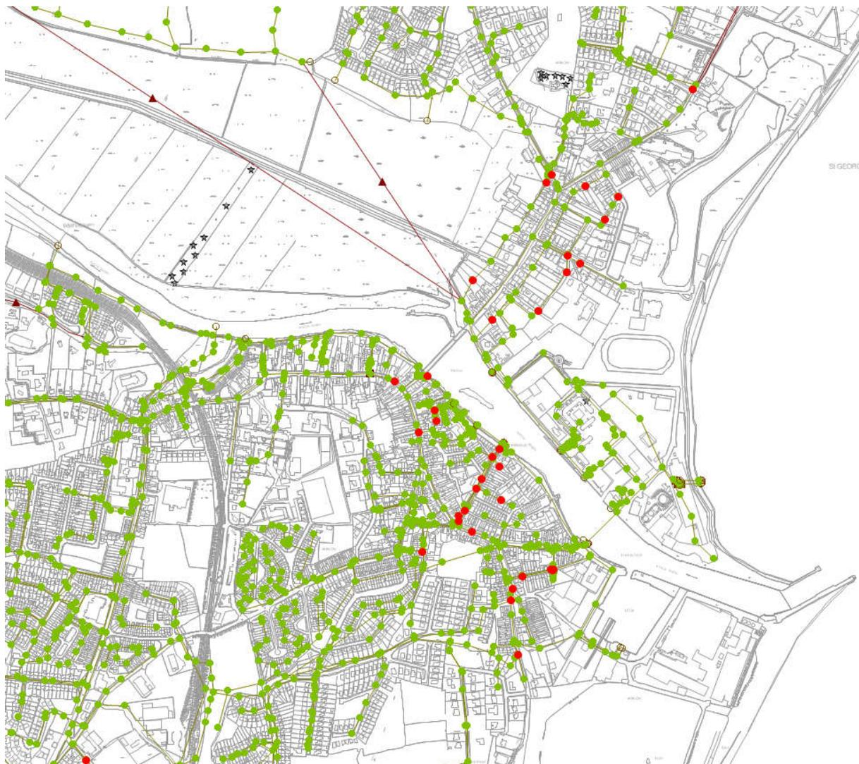
**Figure 6** Predicted flooding locations with flood volume > 25 m<sup>3</sup> with all pumps down for M30\_60 & MWSH with CC
