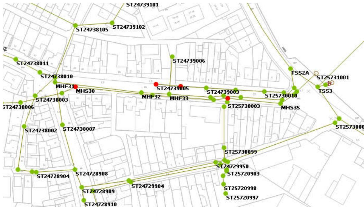
**Figure 4** Scenario 2 - Predicted flooding locations with flood volume > 25 m<sup>3</sup>
