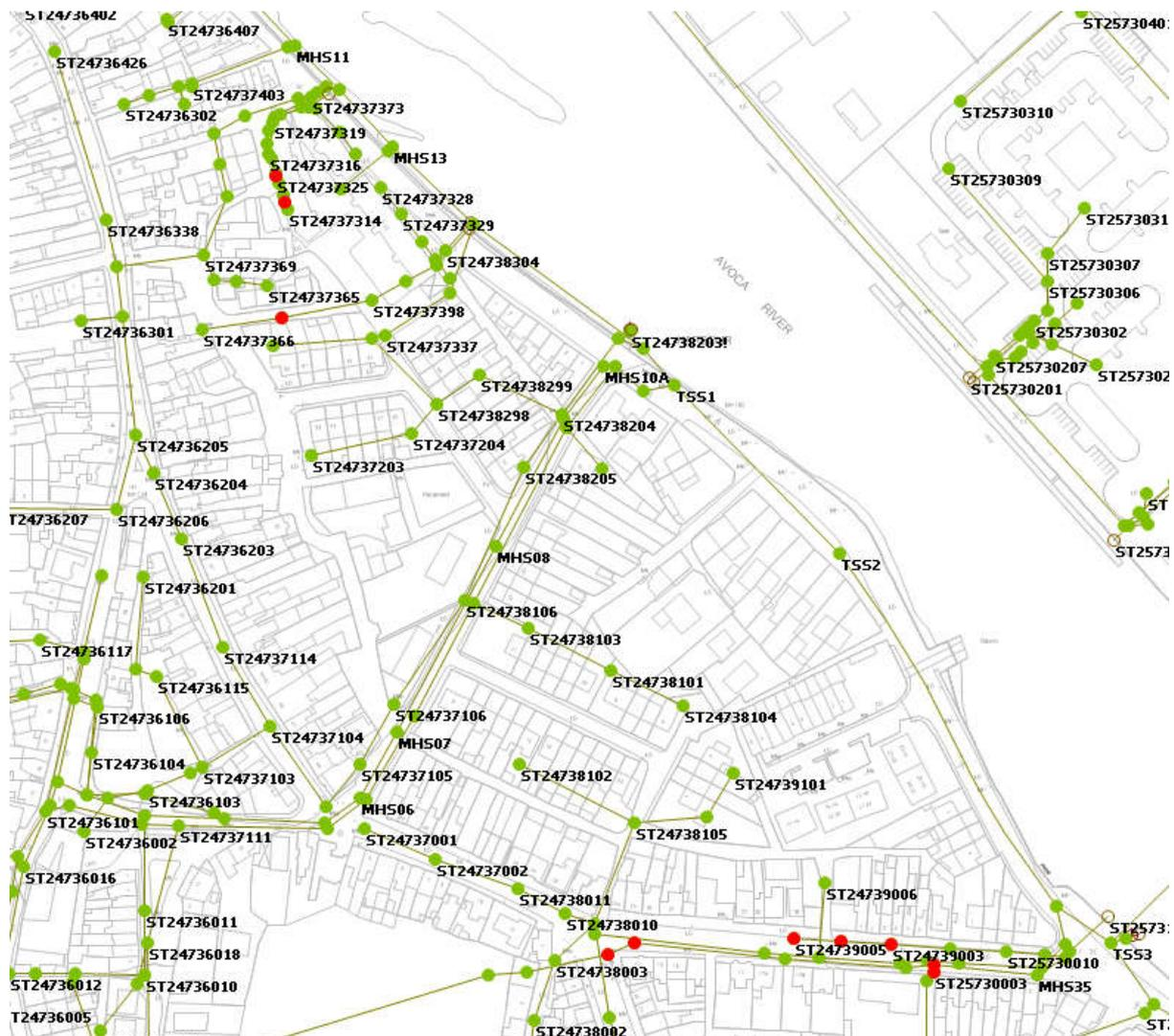
**Figure 5** Scenario 3 - Predicted flooding locations with flood volume > 25 m<sup>3</sup>
