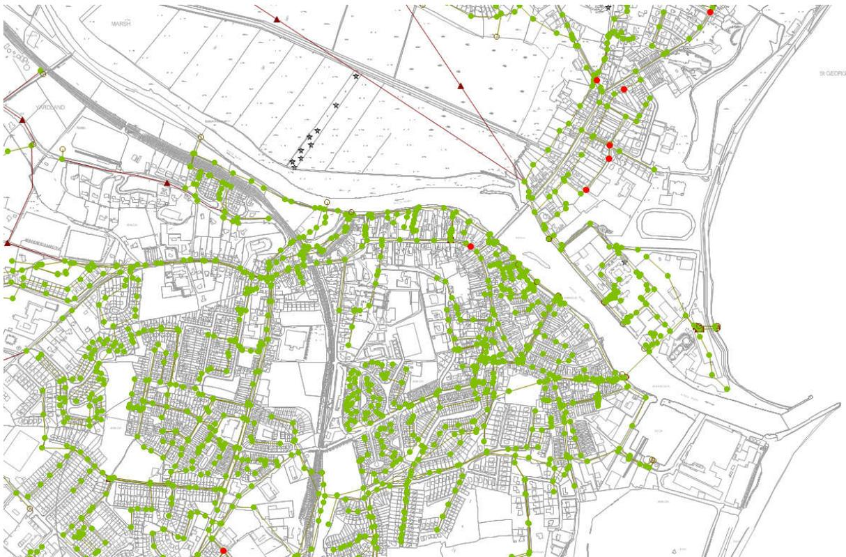
**Figure 7** Predicted flooding locations with flood volume > 25 m<sup>3</sup> with all pumps down for M30\_60 & No tide
